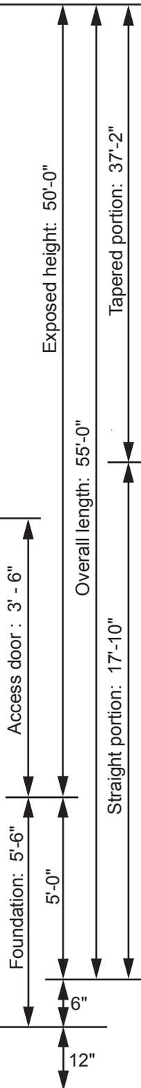
All shafts with overall length of more than 38'-6" are shipped in two sections.
