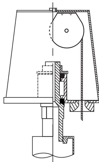
Revolving non-fouling internal halyard truck, cast aluminum body, 26 stainless steel ball bearings, and 2-1/2" diameter plated steel sheave.
