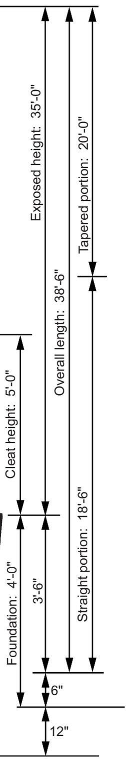
All shafts with overall length of more than 38'-6" are shipped in two sections.
